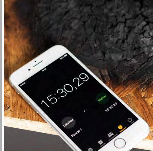
15-minute exposure to flame only chars surfaces.
