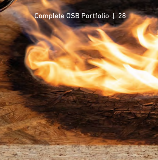
When exposed to flame, SWISS KRONO OSB/3 stop fire EN300 chars to form a fire-inhibiting layer.
